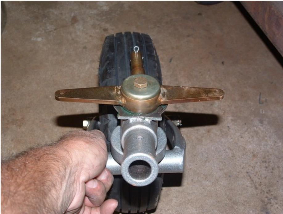
Left– the angle that the rod stinger goes into the tail wheel is determined by angle out of aircraft and desired angle of king pin at full gross. (vertical or slightly toe ahead)
