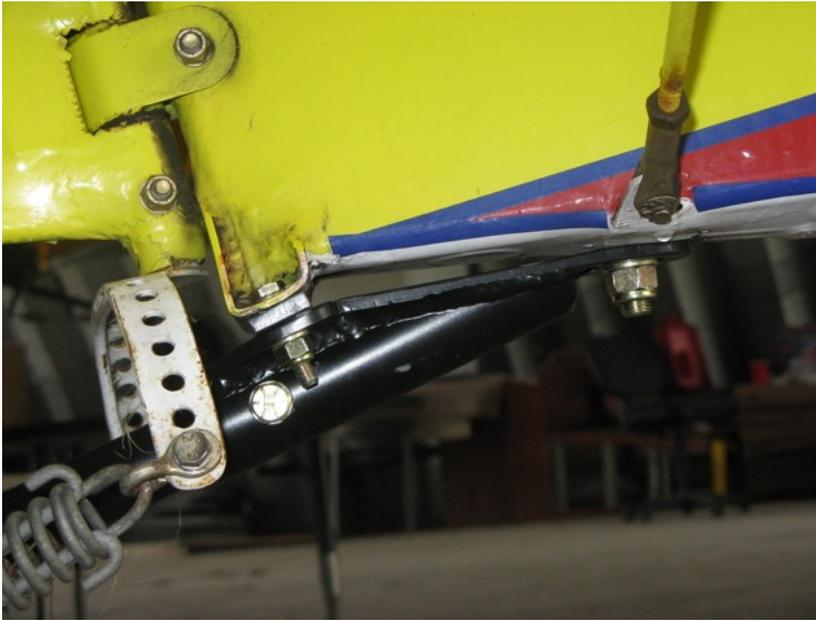
Left– showing adapter bolted onto same location of flat spring. This is a welded unit with female socket.
