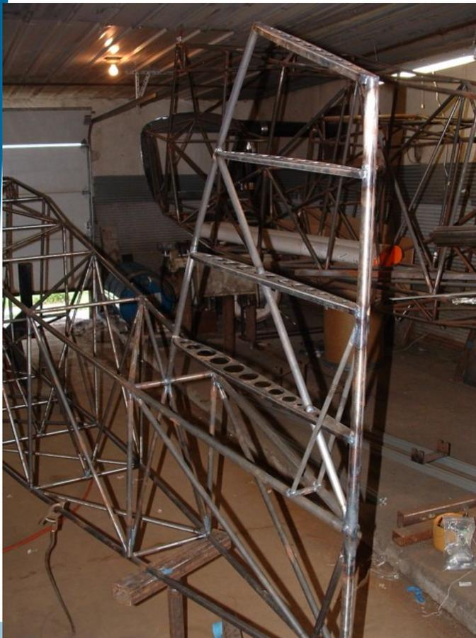
(left view) Finished V Stab with ribs in place. Offset on bottom, centered top. That is your choice and ribs will allow either centered or offset top. Don't forget your brace tube as you put into place.
