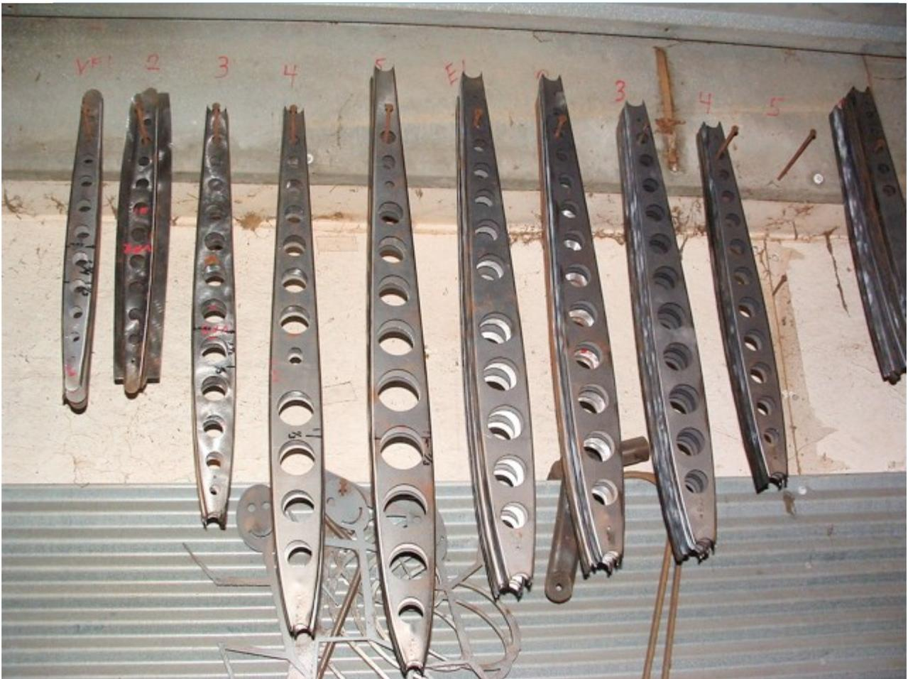
Filled in ends for ribs that are located on ends of H-stabs or elevator . See upper left. All holes to the max allowed producing the lightest yet strong ribs. The stick men in the background like them too!
