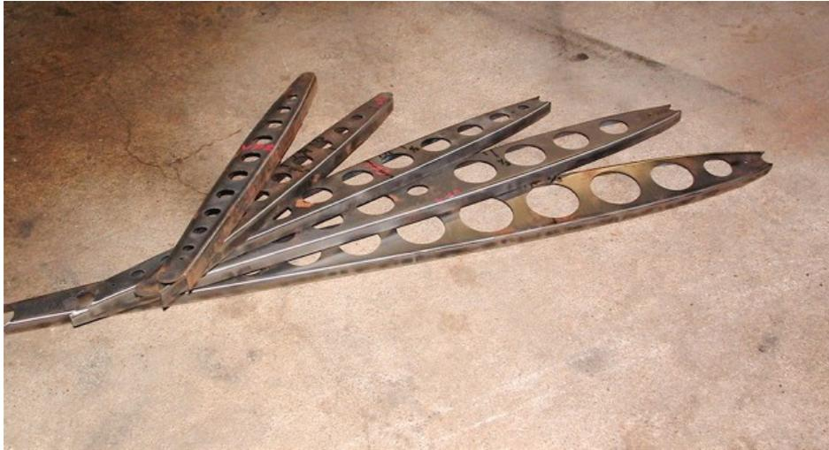
Peened and hammered over steel form blocks for smooth sides and nice radius edges. NO flutes on sides. This heat and shrink method gives the strongest rib shape possible. All lay very flat as shown here.
