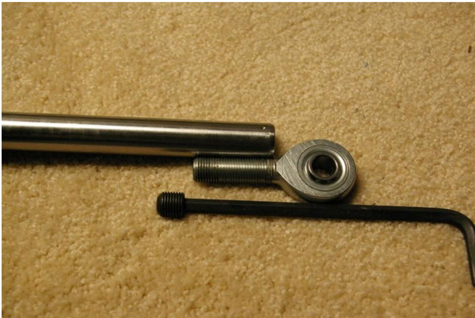
Note: the hole has been tapped .600" deeper than the rod end threads. The special loc-tite sealant was inserted down the tube via a straw for the plug. This requires a cleaning process and 24 hr. dry period for the sealant to set up. More details on next pages.
