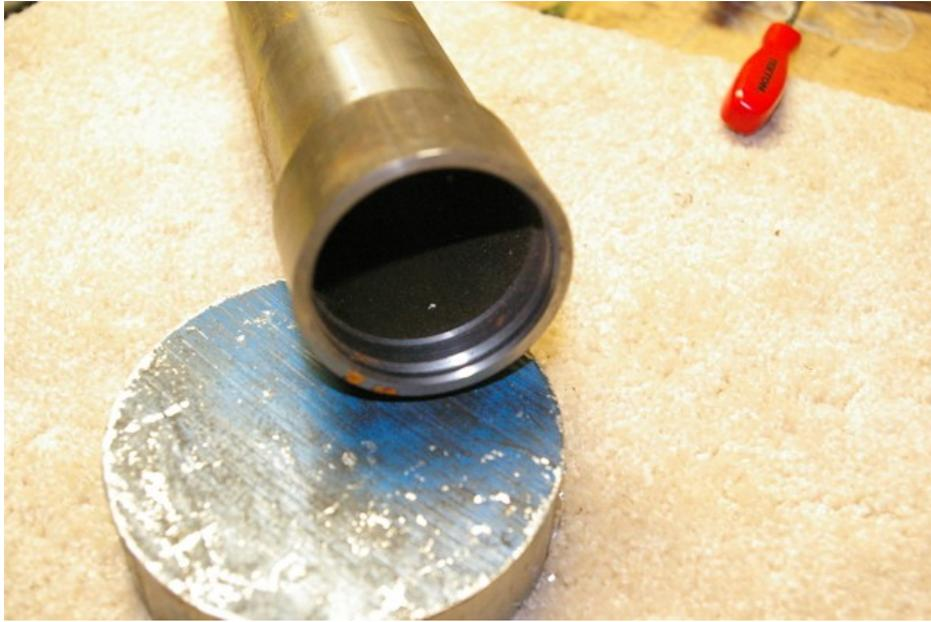
The ramp to the tube needs to also be chamfered, as this location is where the o-rings slide in (piston and the bronze cap ring) We can't risk cutting those after all this work has been done.
